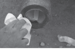
Clean Excess Paste From Mold
